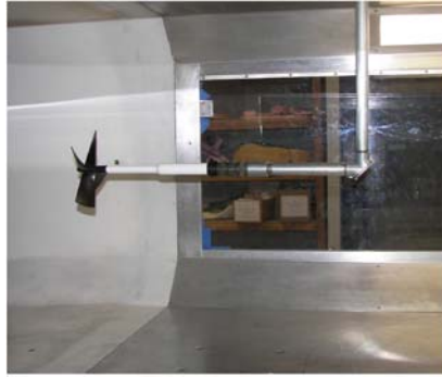
Figure 6.10. Propeller anemometer in wind-tunnel calibration facility.
