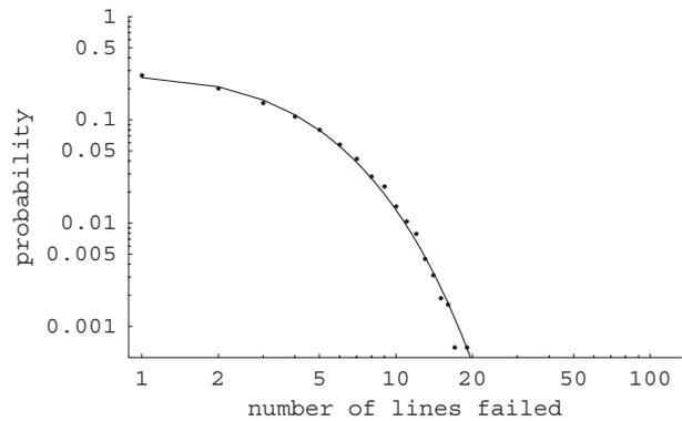
**Fig. 4.** IEEE 118 node test system with loading factor 1.0. Probability distribution of line outages estimated with branching process (solid line) compared with OPA empirical distribution (dots). Reprinted with permission from Reference 29. © 2007 IEEE.
