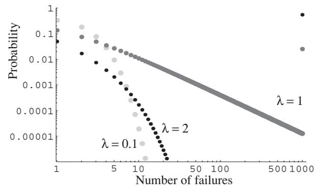
**Fig. 1.** Log-log plot of probability distribution of total number of failures  $Y$  in branching process model with saturation at  $S = 1,000$  failures for three values of propagation  $\lambda$ . The distribution has an approximate power-law region at criticality when  $\lambda = 1$ . The probability of 1,000 failures is 0.025 for  $\lambda = 1$ , and 0.797 for the supercritical case  $\lambda = 2$ .
