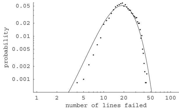
**Fig. 5.** IEEE 118 node test system with loading factor 1.3. Probability distribution of line outages estimated with branching process (solid line) compared with OPA empirical distribution (dots). Reprinted with permission from Reference 29. © 2007 IEEE.
