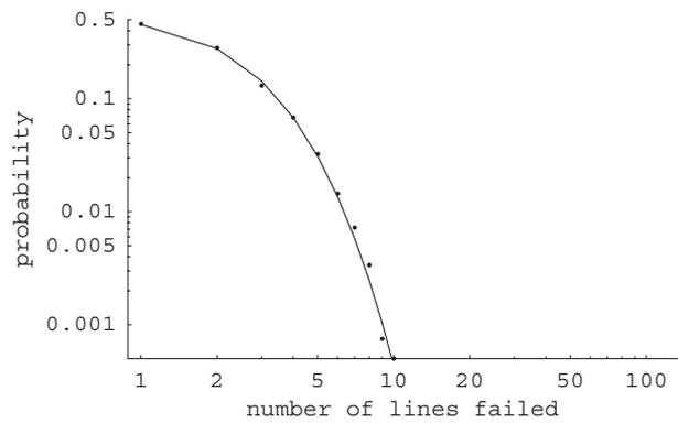
**Fig. 3.** IEEE 118 node test system with loading factor 0.9. Probability distribution of line outages estimated with branching process (solid line) compared with OPA empirical distribution (dots). Note the log–log scales. Reprinted with permission from Reference 29. © 2007 IEEE.
