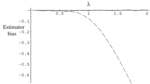
**Fig. 2.** Bias of estimator  $\hat{\lambda}_s$  (solid line close to horizontal axis) and bias of standard estimator  $\hat{\lambda}_n$  (dashed line) plotted against  $\lambda$  from saturating branching process with  $\theta = 1$  and saturation  $S = 20$ . The bias is estimated from 1,000 samples of the estimator for  $K = 50$  nonzero cascades.
