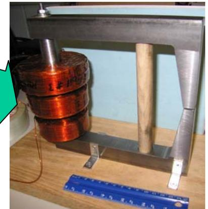
...we decided to take matters in to our own hands and build a benchtop 1 Tesla electromagnet. Sufficient for the ferrite magnets, we'll need to send out the higher-energy samples for magnetization.
