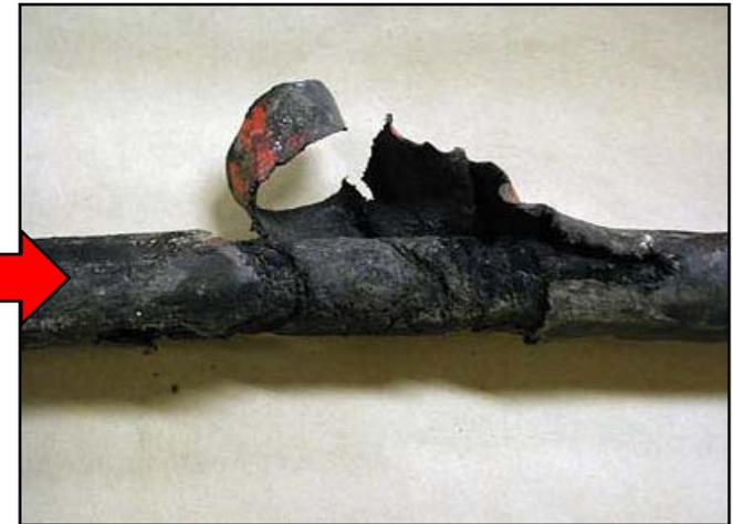
**Failure Mechanism:** Microvoids and channels form in insulator due to electrical forces, water seeps in and fills them, forms tree-like conducting structure. Ultimately a high-powered brief arc occurs producing damage pictured above.
