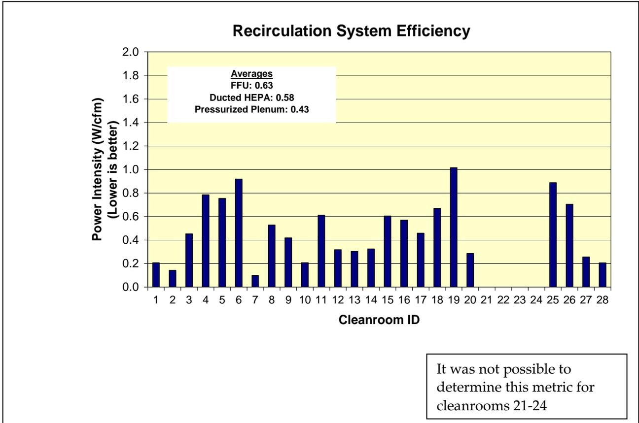
**Figure 3. Cleanroom recirculation air system efficiency**
