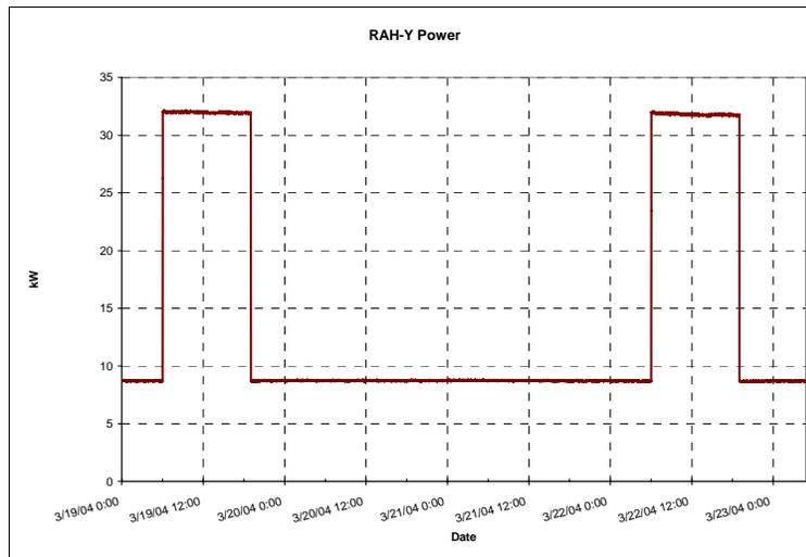
**Figure 1. Recirculation fan energy savings during setback at facility 1.**
