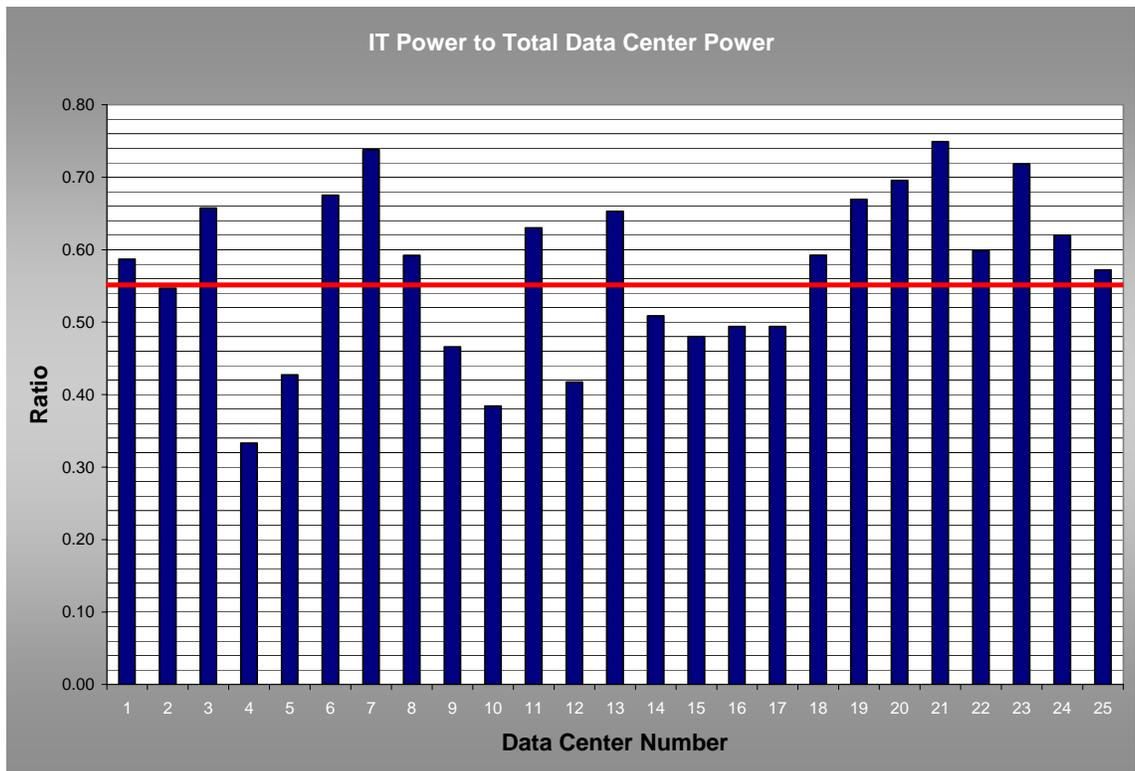
**Figure 5. Ratio of IT power to total data center power**
