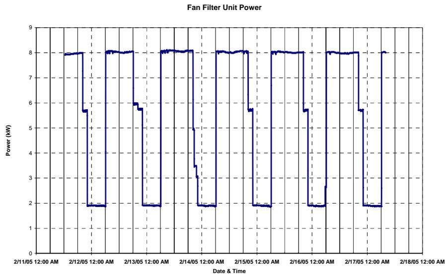
**Figure 2. Recirculation fan energy savings during setback at facility K.**
