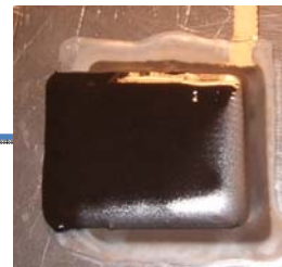
Dispenser printed capacitor (C.Ho)
