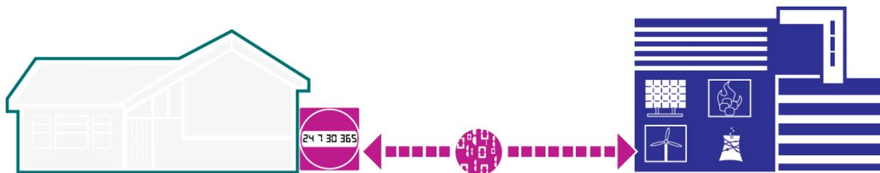
A smart meter (in magenta, attached to the side of the house) collects, stores, and transmits short-interval meter data from the home to the utility (drawn in blue). Smart meters also facilitate two-way communications between the meter and the utility. Energy usage information is depicted as a bidirectional arrow composed of discrete square elements.
