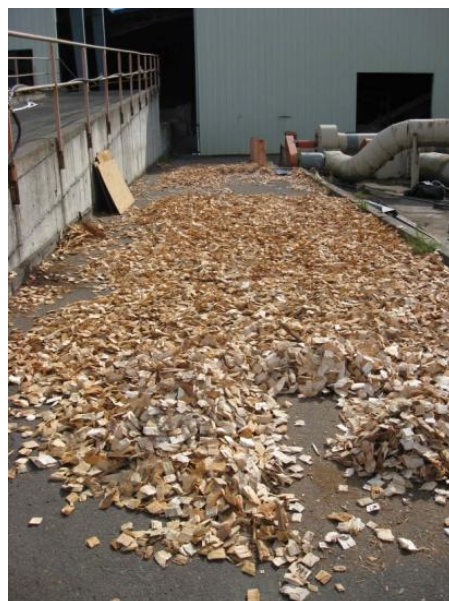
Figure 4. Air-dried hog fuel used in the TSY-Peak biochar system Photo Credit: Matt Delaney
