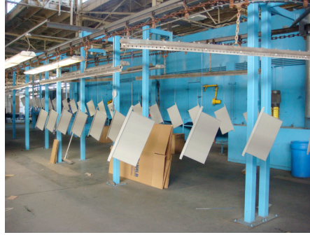
Pressure plates being powder-coated in the paint factory
