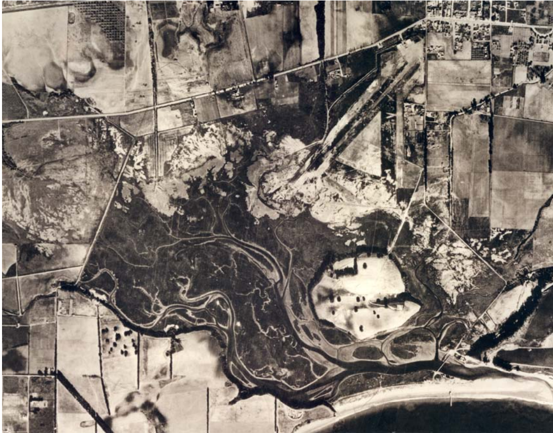
Figure 2.23: Aerial Photograph of the Santa Barbara Airport Site in 1938. At that time, there was only a small dirt runway that was constructed to fill the slough and create three runways for Marine Corps Air Station Santa Barbara, as part of an Army Corps of Engineers project.
