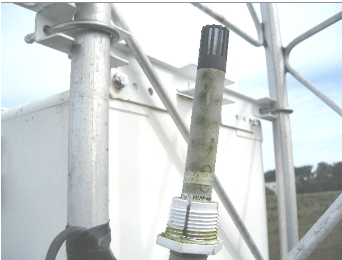
Figure 34. Point Reyes National Seashore RCA Building site. Radiation shield has been removed to reveal mildew and organic film covering portions of the support for the temperature and humidity sensors, which are located in the dark gray slotted area near the top of the photo.
