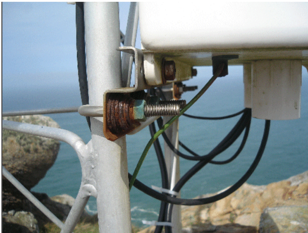
Figure 35. Point Reyes Lighthouse Rock station, showing corrosion of steel bolt after 18 months of exposure to salt. Site is 526 feet directly above the Pacific Ocean.
