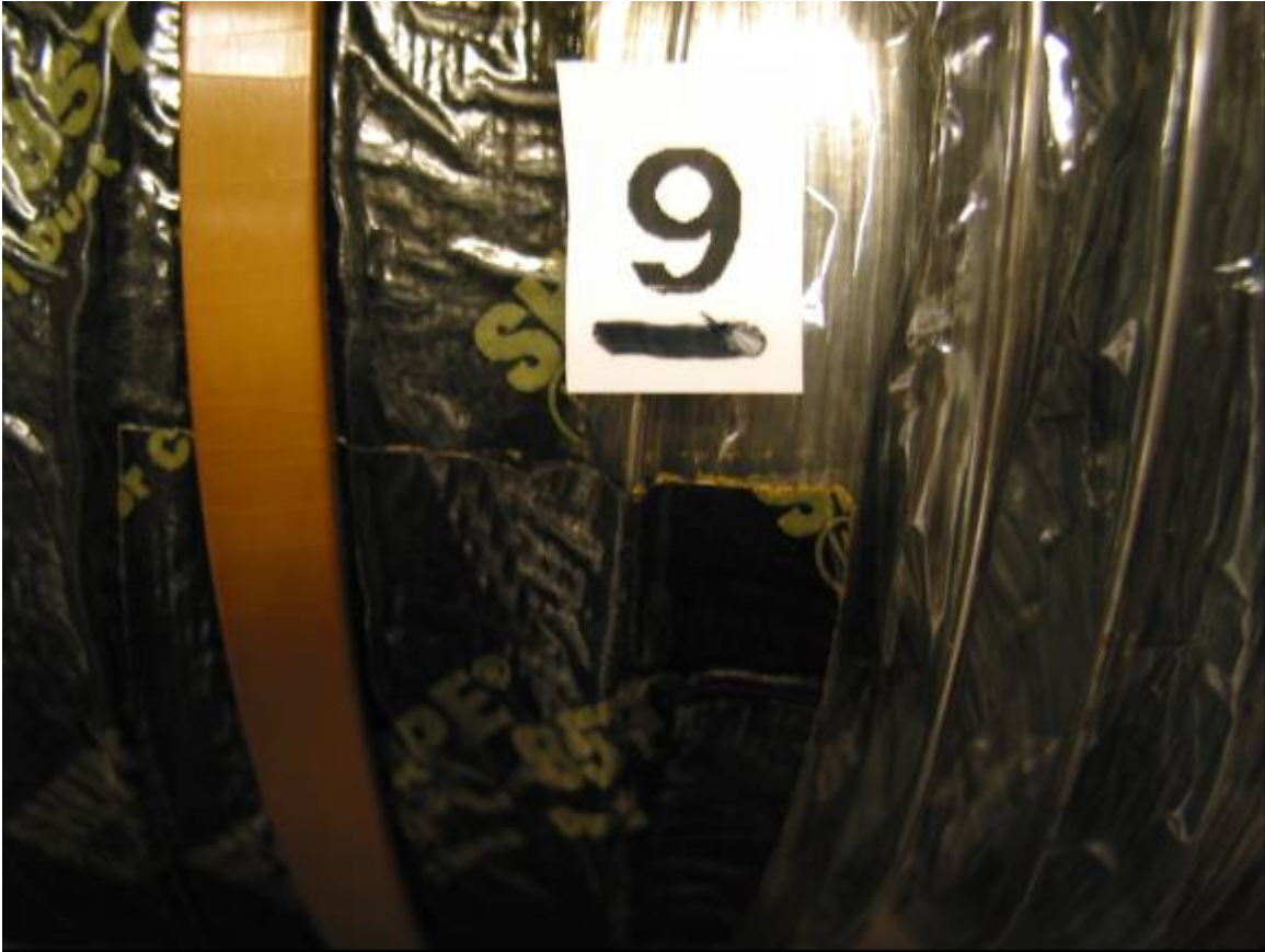
Figure A11. Sample 9. This sample shows almost no shrinkage or delamination.
