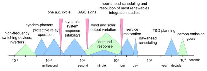
Figure 1. Time scales in electric grid operation.
