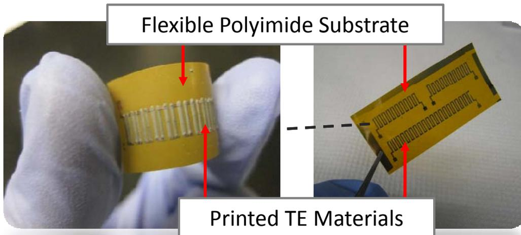
Leg Dim.: 5 mm Length, 500  $\mu\text{m}$  width, 200  $\mu\text{m}$  thick
