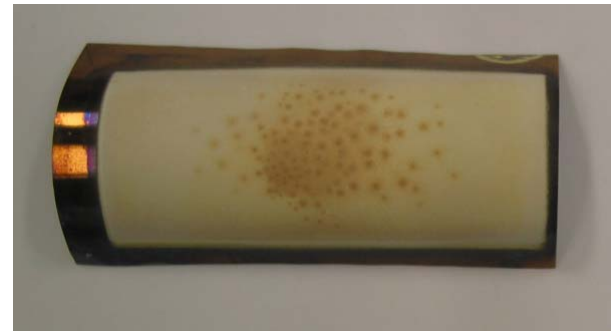
Sputtered PZT film on 25 \mu m steel shim
