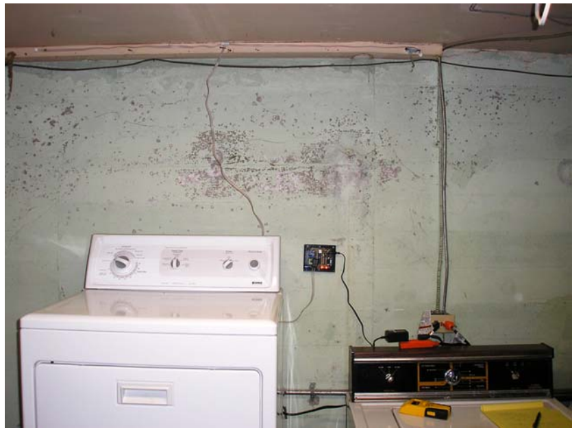
Figure 10.5. a) Data logger mounted below existing thermostat; b) Data logger mounted in basement next to washing machine, seen with dipole antenna mounted near ceiling
