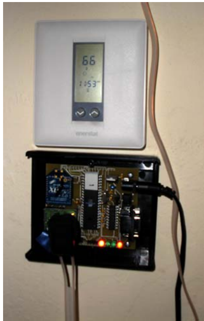
Figure 10.5. a) Data logger mounted below existing thermostat; b) Data logger mounted in basement next to washing machine, seen with dipole antenna mounted near ceiling
