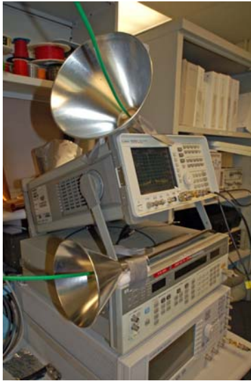
Figure 1. The in-lab single green insulated wire GW setup. (left) Photograph showing the wire (i), launch (ii) and receive (iii) cones. (right) Schematic of the GW setup.
