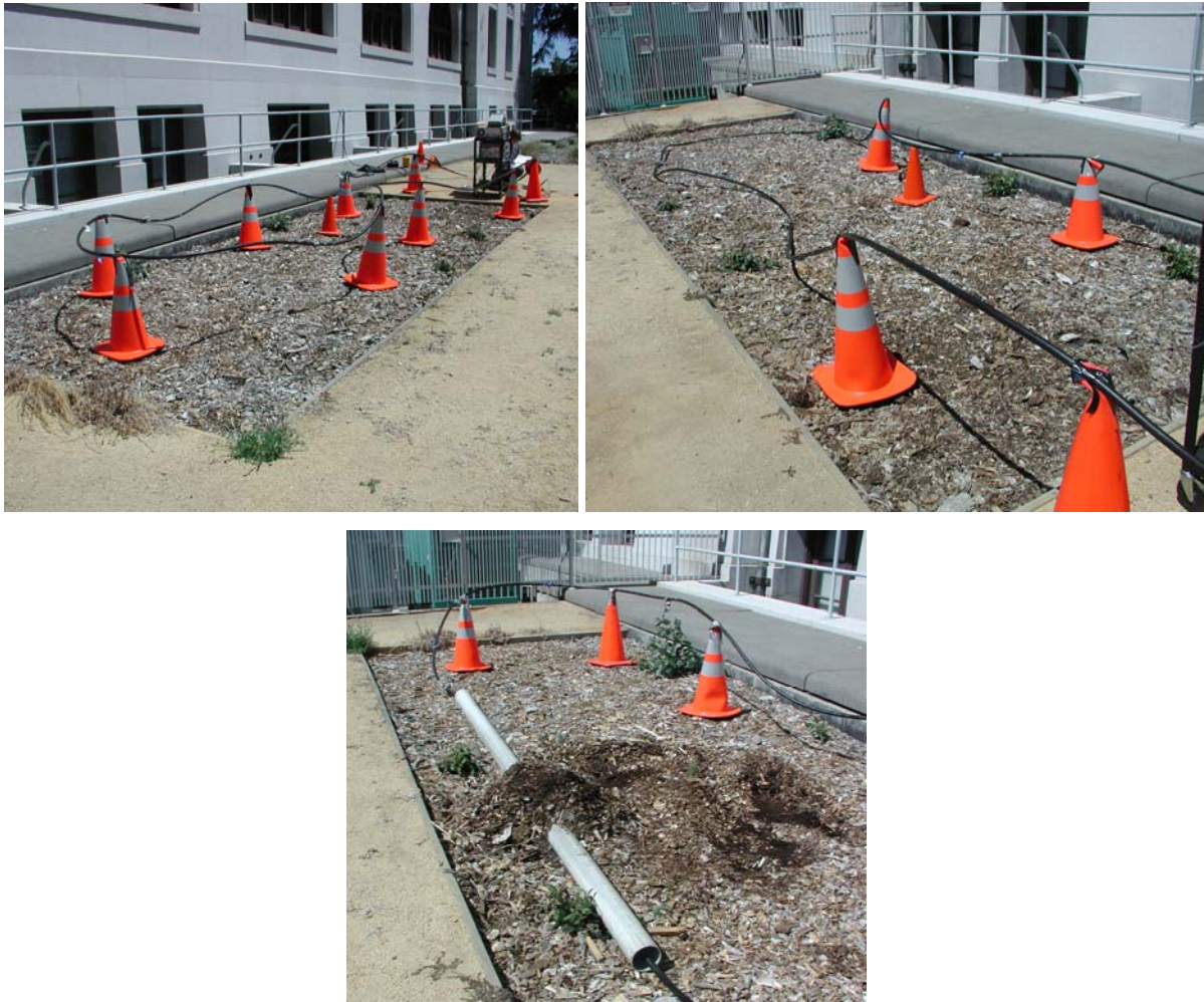
Figure 3. The 64 feet outdoor underground cable GW setup. The cable was at times completely ( top-left ) or partially ( top-right, bottom ) supported by 29-inch tall plastic traffic cones.
