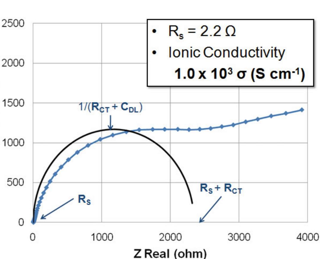
Nyquist plot of impedance spectroscopy of PVA-KOH-H₂O film between zinc electrodes
