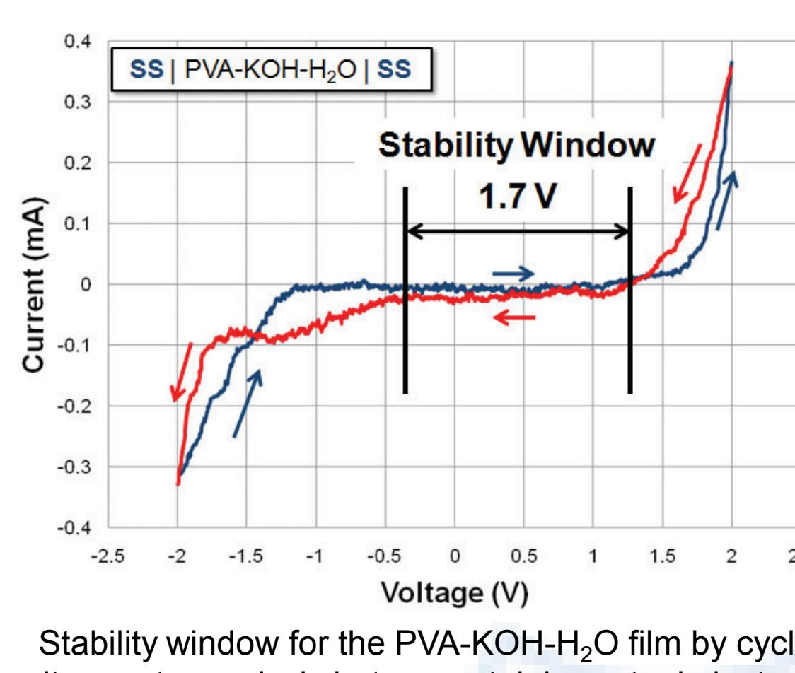
Stability window for the PVA-KOH-H₂O film by cyclic voltammetry analysis between stainless steel electrodes
