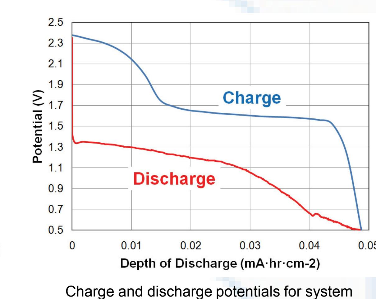
Charge and discharge potentials for system after 50 cycles
