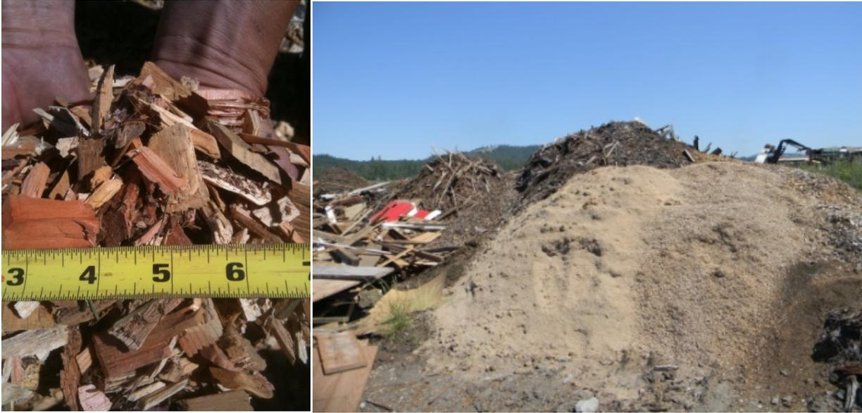
**Figure 3.** Wood waste used in the TSY-Peak biochar system. Left is the hog fuel used to power the gasifier. Right is the waste biomass currently left to rot in the log yard, which feeds the pyrolytic retort.
