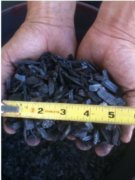
Figure 5. Biochar product produced by the TSY-Peak system.
