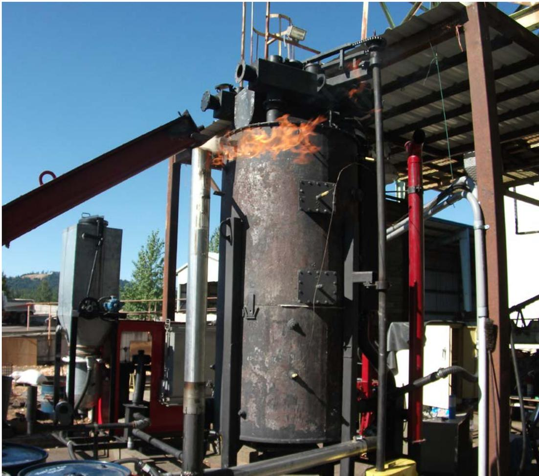
**Figure 2.** Fluidyne Gasifier (left background, metallic surface) and pyrolytic retort (right front, black paint) in the log-sorting yard of Thompson Timber/Starker Forest, Philomath OR.
