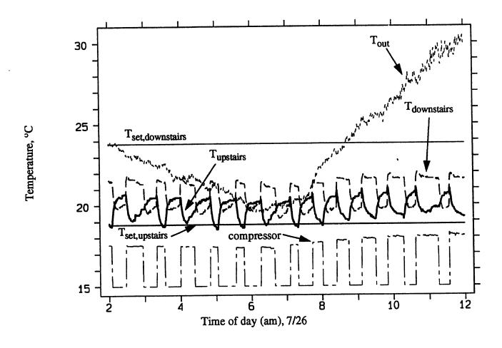
FIGURE 2. Upstairs cooling only, room temperature response and outside temperature, °C, rescaled compressor power demand showing system operation.  $T_{\text{set,up}} = 18.8 \text{ °C}$ ,  $T_{\text{set,down}} = 23.8 \text{ °C}$   $T_{\text{up}} = 19.8 \text{ °C}$ ,  $T_{\text{down}} = 20.7 \text{ °C}$
