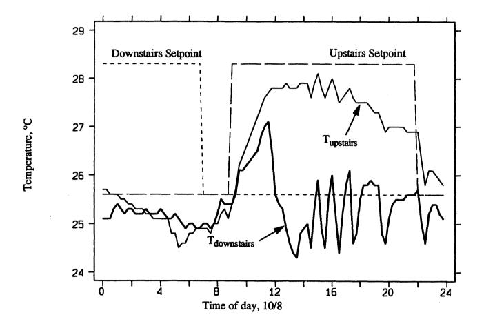
FIGURE 3. Downstairs cooling only, room temperature response, upstairs and downstairs thermostat schedules, average temperatures between 9 am and 10 pm:  $\overline{T}_{up} = 27.4$  °C,  $\overline{T}_{down} = 25.5$  °C
