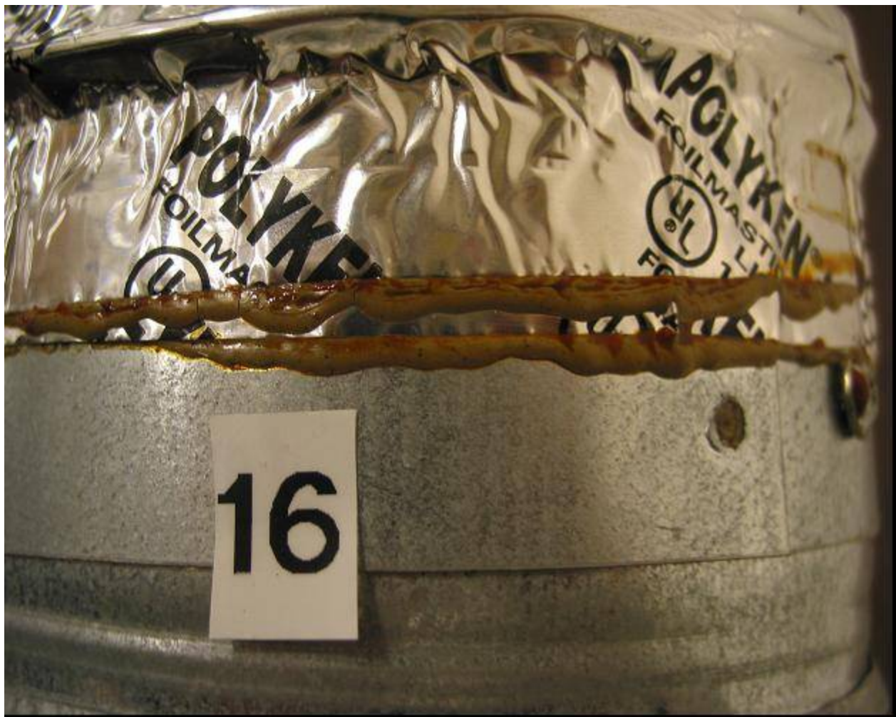
Figure A19. Sample 16. This sample shows oozing of the adhesive at the tape edges.
