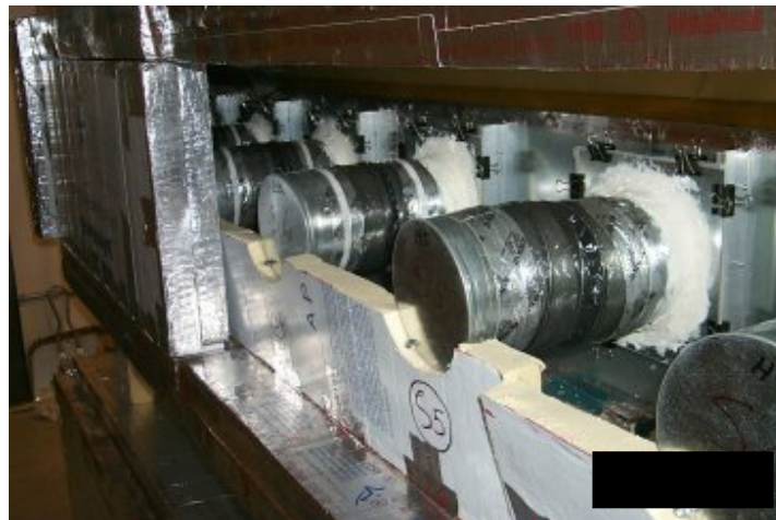
Figure 4. One chamber of the high temperature aging test apparatus.
