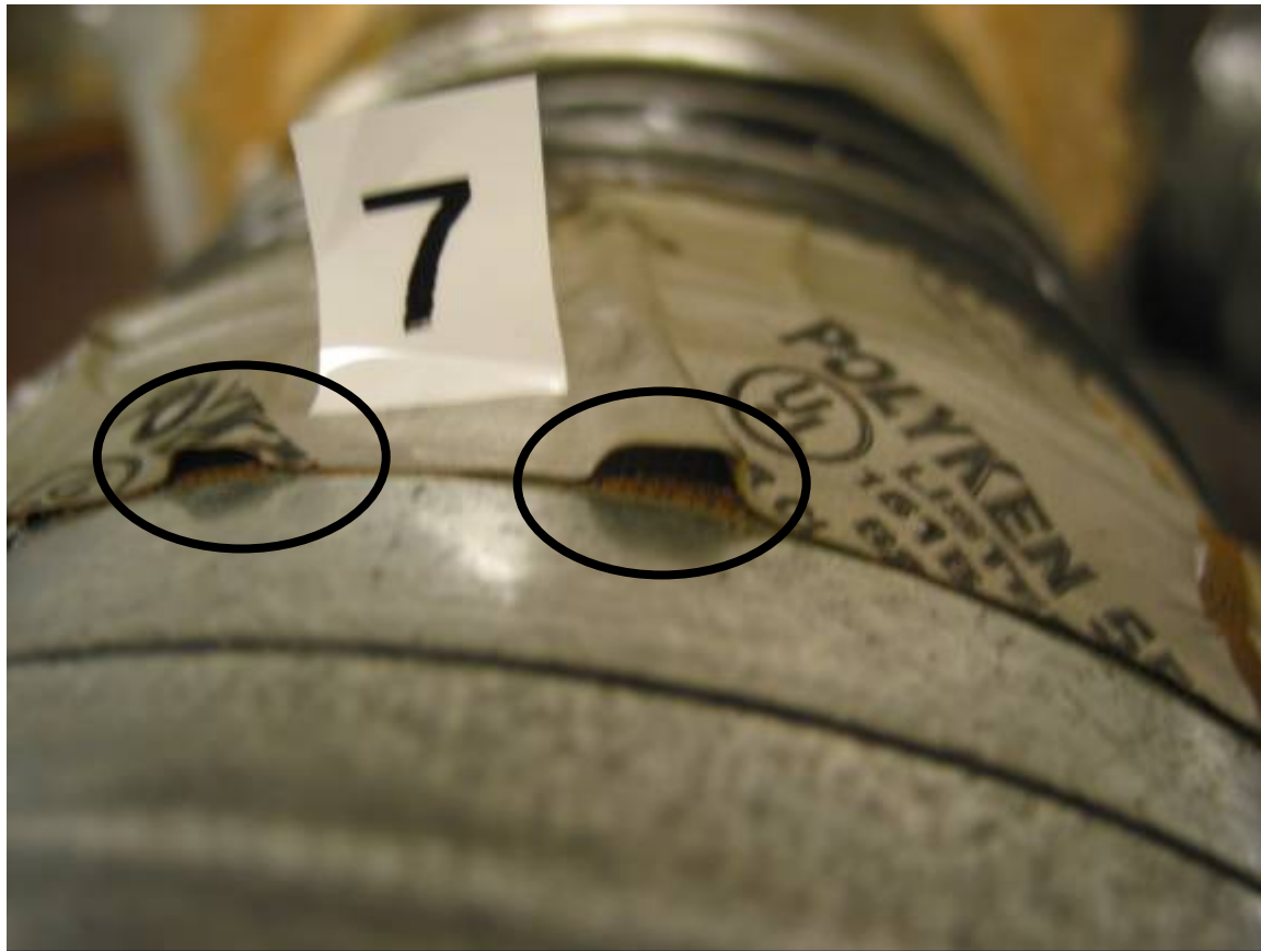
Figure A8. Sample 7. The edges of the tape have lifted off the duct surface in large wrinkles.
