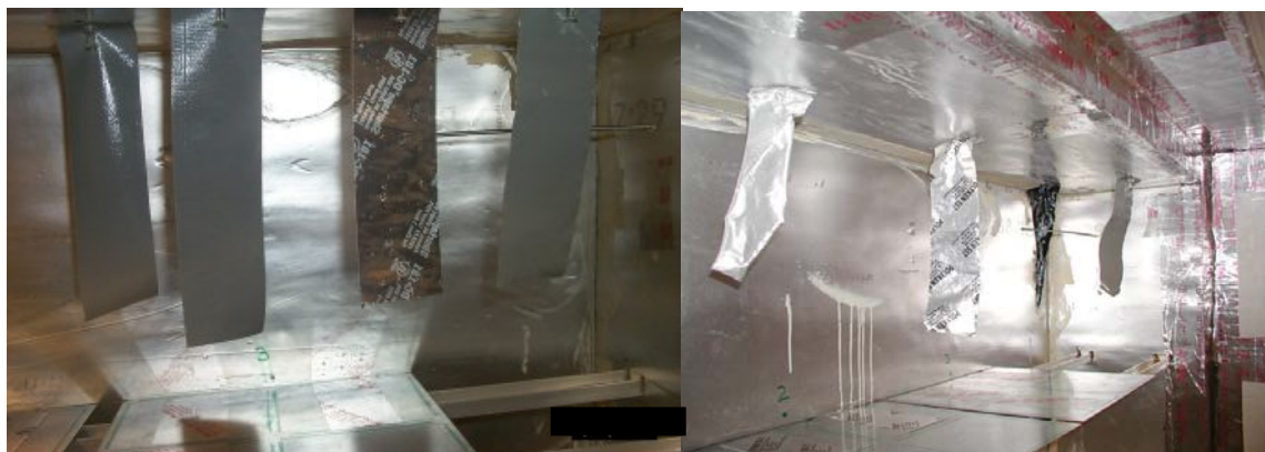
Figure 9. Hanging specimens of Tapes 1 to 4 in the high temperature baking apparatus before testing (left) and after three weeks of testing (right).
