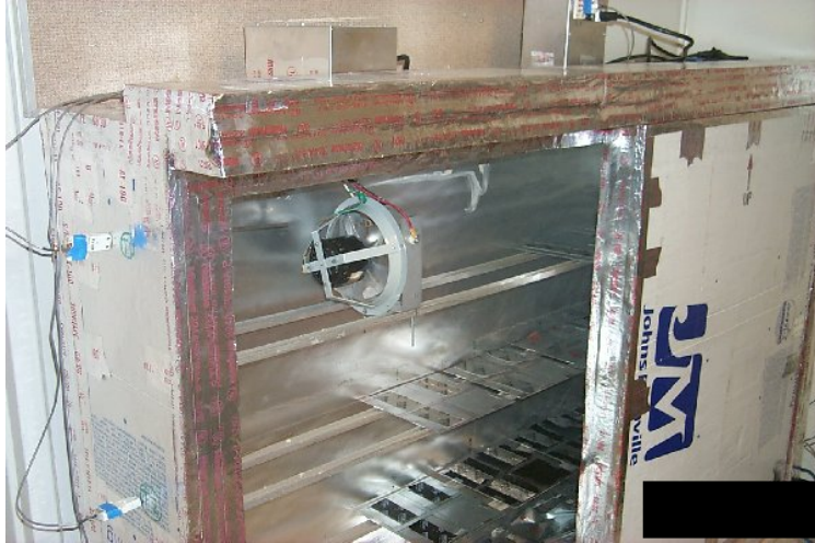
Figure 7. The high temperature baking apparatus.
