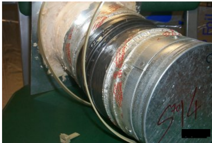
Figure 14. Failed plastic strapping on one of the flexible core to sheet metal collar specimens after four months of aging.
