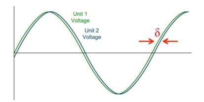
the small phase angle  $\delta$  between different locations on the grid drives a.c. power flow
