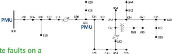
Can angle help locate faults on a long feeder?
